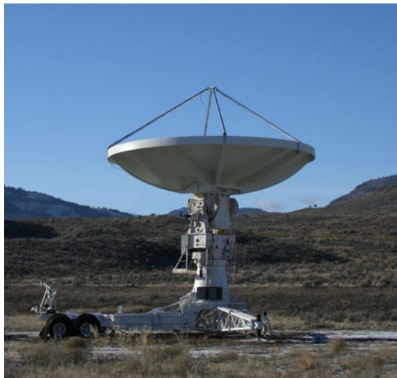
Prototype design of a composite antenna at DRAO in Penticton, Canada. The 10-m dish of this composite antenna was placed on the MV-1 antenna mount (formerly at Yellowknife).
