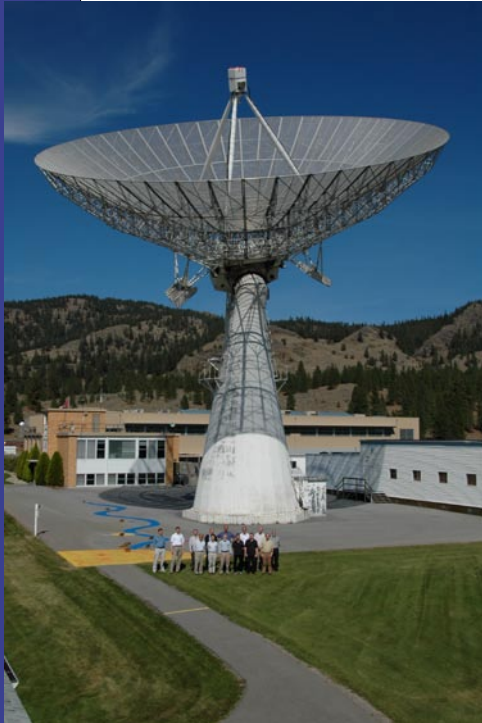
The Directing Board in front of DRAO's 26-m antenna. This antenna was involved in the first VLBI experiment on a long baseline (with Algonquin) successfully yielding fringes in 1967.
