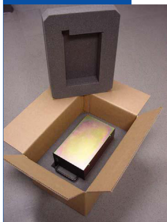
(top) Mark 5 module (“8-pack”) populated with eight disks. (below) Mark 5 module with shipping covers installed is readied for shipment in tailor-made shipping box.
