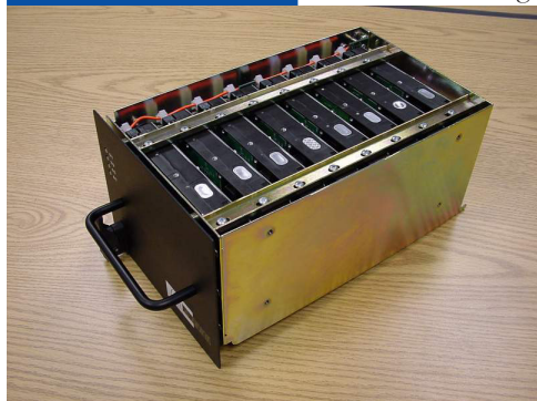
(top) Mark 5 module (“8-pack”) populated with eight disks. (below) Mark 5 module with shipping covers installed is readied for shipment in tailor-made shipping box.
